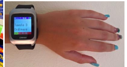
Wrist pager with color display, rechargeable lithium battery
